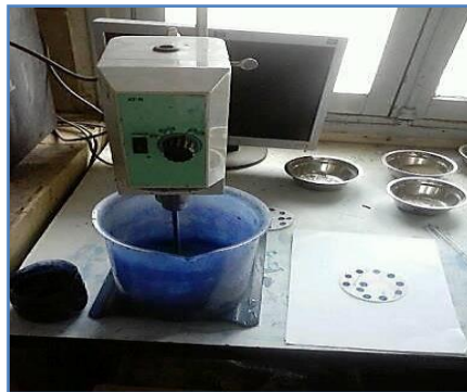
Figure 11.Methylene blue test equipment.
