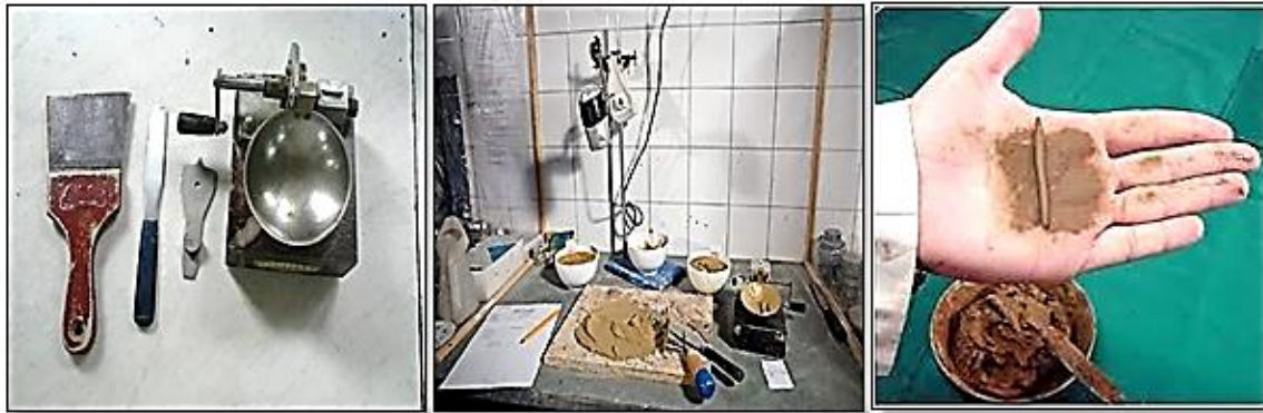
Figure10. Apparatus for the determination of Atterberg limits.
