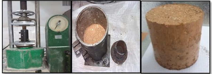
Figure 15. Sample preparation by static compaction (to determine water content).
