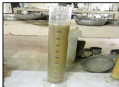
Figure 12. Reading test grain density.
